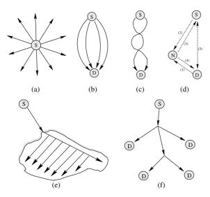
Fig. 1. Trajectory based flooding, routing and discovery.
