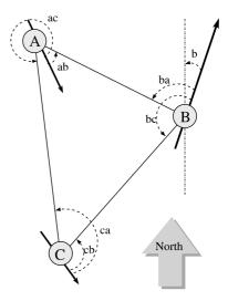
Fig. 2. Nodes capabilities: measuring angles, ranges, orientation.
