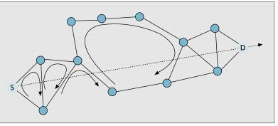
**Figure 4.** *The FACE algorithm routes around obstacles using the lefthand rule.*
