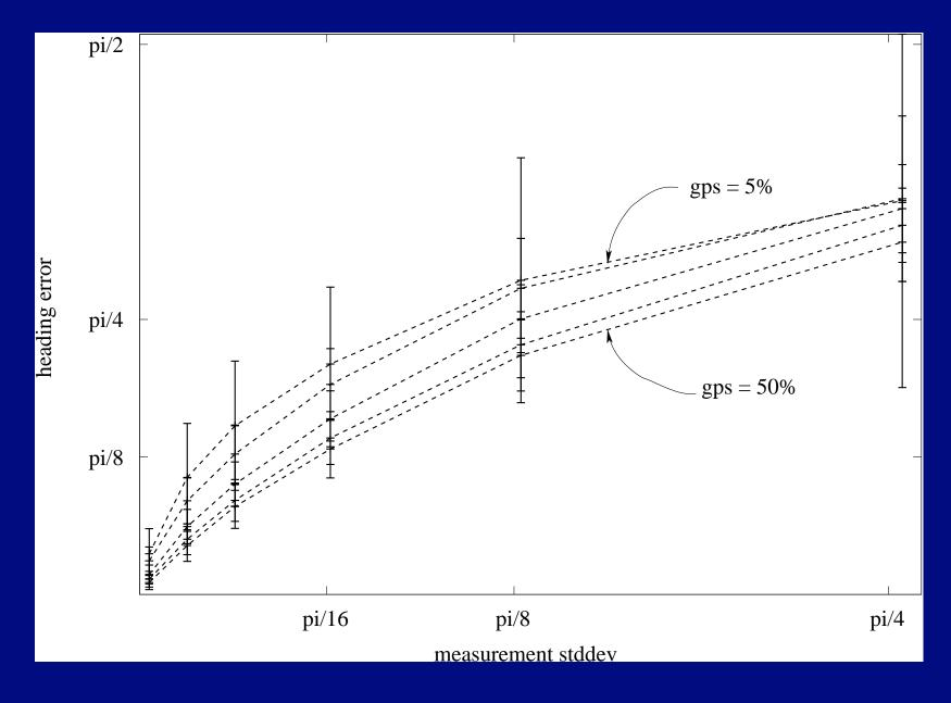
$\bigcirc$  Heading error – double of the bearing error
